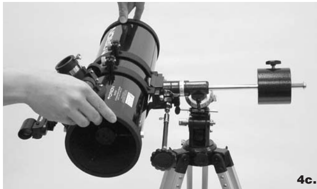
Figure 4. Proper usage of the equatorial mount requires the telescope tube to be balanced on both the R.A. and Dec. axes. (a) With the R.A. lock knob released, slide the counterweight along the counterweight shaft until it just counterbalances the tube. (b) When you let go with both hands, the tube should not drift up or down. (c) With the Dec. lock knob released, loosen the tube ring lock clamps a few turns and slide the telescope forward or back in the tube rings. (d) When the tube is balanced about the Dec. axis, it will not move when you let go.
