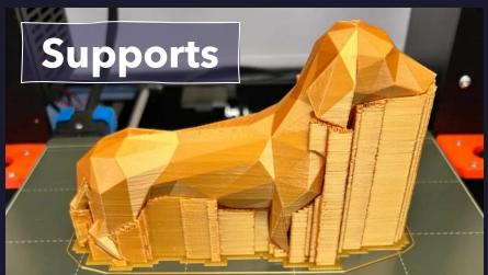
**Supports:** Very important for prints with overhangs, especially over **45 degrees**, because you cannot print in midair.
